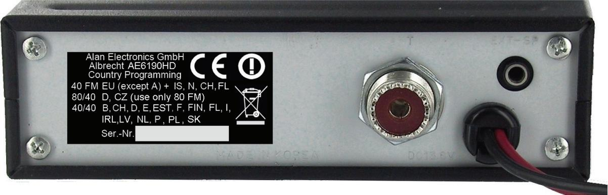
Brand Plate with country switching decription      Antenna socket 50 Ohms PL-259 Standard      DC power cable 13.2 V
