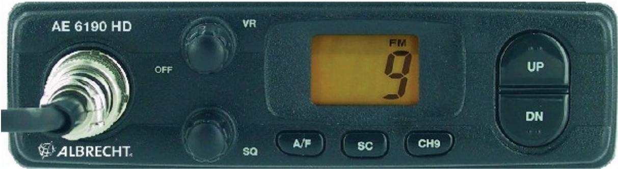
6 pin MIC socket      Squelch      AM -FM      Scan switch      CH 9      Channel Down key
